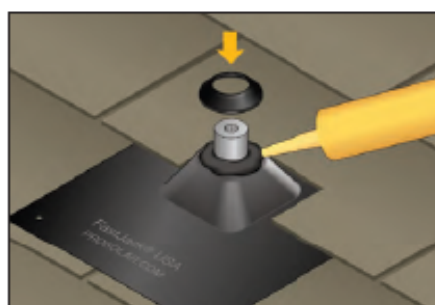
Step 7: Apply 1/4" bead of sealant (Geocel 4500) and compress with Aluminum collar.
