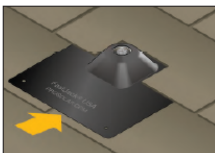
Step 5: Slide FastJack® flashing under shingle
