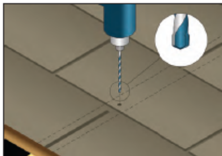
Step 1: Drill rafter pilot hole with 3/16" carbide bit
