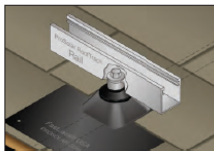
Step 9: Attach ProSolar RoofTrac® rail and clamps
