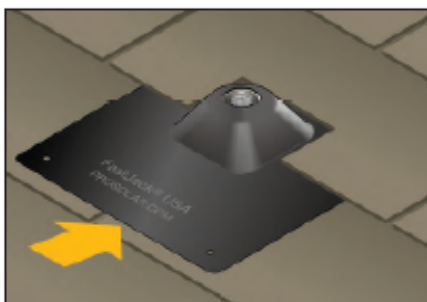
Step 5: Slide FastJack® flashing under shingle
